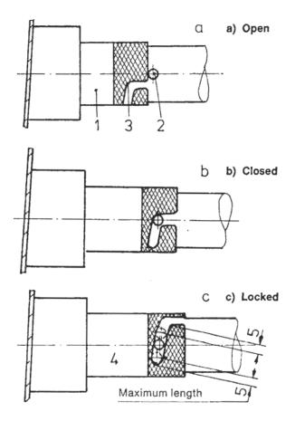
After connecting the quick lock couplings make a visual check that the collar is extended forward over the bearing far enough for the safety pin to engage. Having engaged the quick locks check that the safety pin cannot be moved without pressing it down. If it cannot be slid without pressing down the controls are properly connected.
