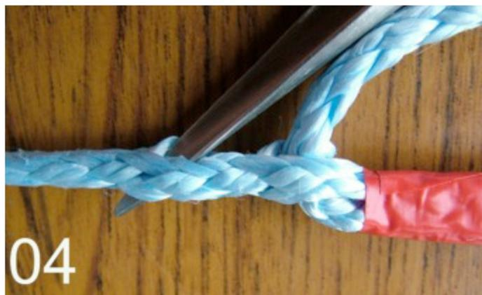
The next step is a fiddly one. When you open up the rope by pushing along its axis you can see little holes where the strands open up. Skip two holes, from the exit point of the first tuck, and push
