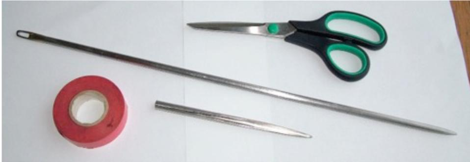
All the tools you need are shown in the picture above. Working from the top we have a sharp pair of scissors, or you can use a sharp knife (it's surprisingly tough to cut), a large darning needle (this was the prototype, and we now use a shorter one), a "fid" – a pointy tubular tool for threading one rope through another, and some ordinary electrician's tape.
