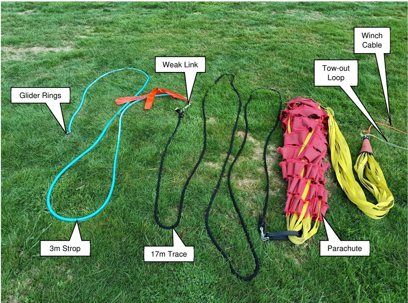
*Pass: Identifies and checks each component on the "glider end" of the cable. Note that some items may be disconnected for tow-out.*
