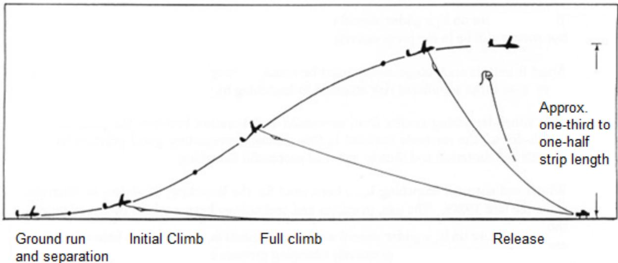
The key requirement in a winch launch is to maintain the correct speed of the glider at all phases of the launch.
