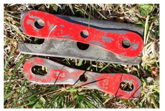
BGA have notified their members that they no longer recommend the double weak link system for winching, due to some incidents and an accident which this may or may not have been a factor. The idea of the double system is that the weak link does eventually wear out and the slotted one will prevent loss of the strop.
